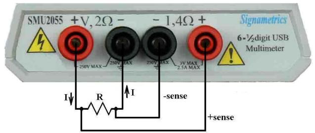
Figure 4-1. The  $I,4\Omega$ + and  $I,4\Omega$ - sense leads should be closest to the body of the resistor when making 4-Wire resistance measurements.
