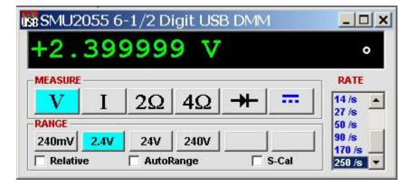
Figure 3-2. The Control Panel. The two main groups include Measurement Function and Range buttons. The Range buttons are context sensitive such that only "240m, 2.4, 24 and 240 appear when in a Voltage Measurement Function is selected, and 2.4m, 24m, 240m and 2.4 appear when a Current Measurement Function is selected, etc.
